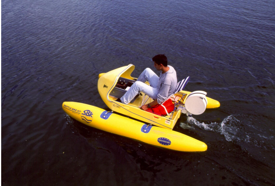
Fig. 1 Hydroxy100, propelled with a 100 W PEFC power pack
