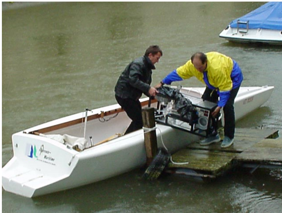
Fig 5 MW-Line Alpha boat propelled by 2 kW PSI PEFC stack
