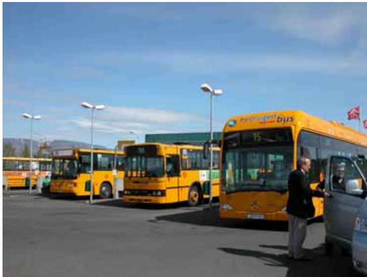
Figure 4.12 The fuel cell buses (furthest right) are taller, heavier and in many ways different from the usual diesel buses in Reykjavik
